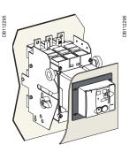
Standard escutcheon for motor mechanism.
