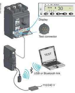
Using the configuration and maintenance module.
