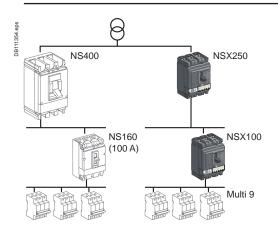
Compact NSX100 with Micrologic for total discrimination with Multi 9 devices rated ≤ 40 A or a C60. Better coordination between protection functions reduces the difference in ratings required for total discrimination.
