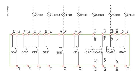
The diagram is shown with circuits deenergised, all devices open, connected and charged and relays in normal position.
