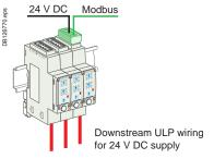
Supply, with the Communication function, via the Modbus
