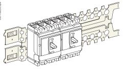
Mounting on a Prisma mounting plate.
