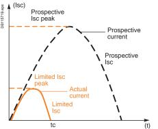
The exceptional limiting capacity of the Compact NSX range is due to the rotating double-break technique (very rapid natural repulsion of contacts and the appearance of two arc voltages in-series with a very steep wave front).
