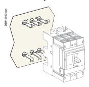
(1) The ØT1 holes are required for rear connection only (for two-pole circuit breakers, the middle holes are not required).
