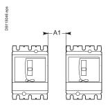
Minimum distance between circuit breaker and front or rear panels
