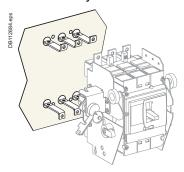
(1) The ØT1 holes are required for rear connection only (for two-pole circuit breakers, the middle holes are not required).
