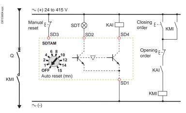
SDTAM wiring diagram with contactor control.
