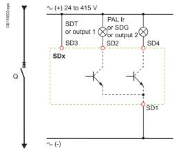
SDx wiring diagram.
