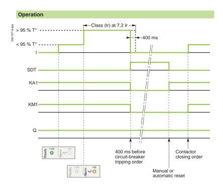
I: charge currentSDT: thermal-fault signal
